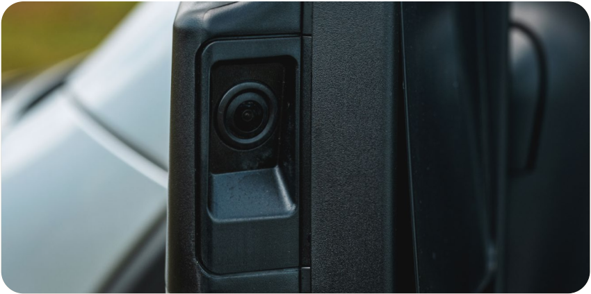
5 Safety sensors and cameras positioned around the exterior of the coach give you comprehensive situational awareness.
